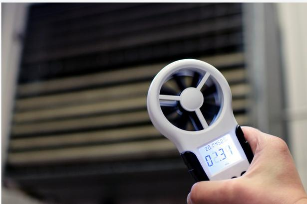
Measuring air flow out of air conditioning outlets is vital to correctly balance the system.
