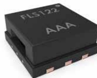
6-pin DFN package 3.5 mm × 3.5 mm footprint < 2 mm overall height
